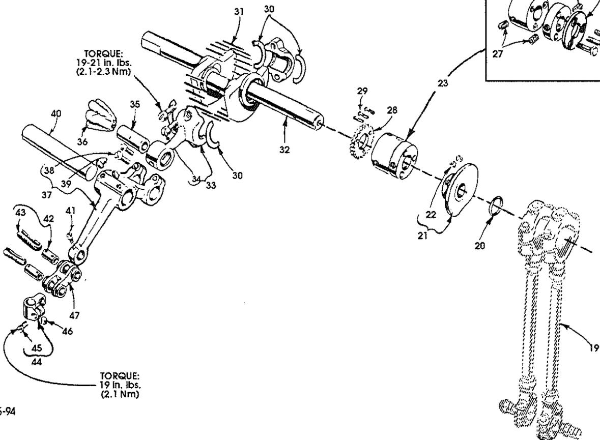
MISCELLANEOUS OILING, NEEDLE LEVER, CRANKSHAFT AND MAIN SHAFT PARTS
