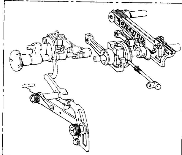
F. 送リ関係 / Feed mechanism / Transportvorrichtung /
