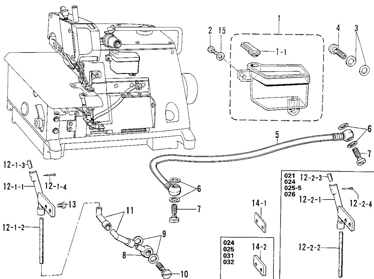
B. 駆動軸関係/Crank shaft mechanism /Kurbelwelle/
