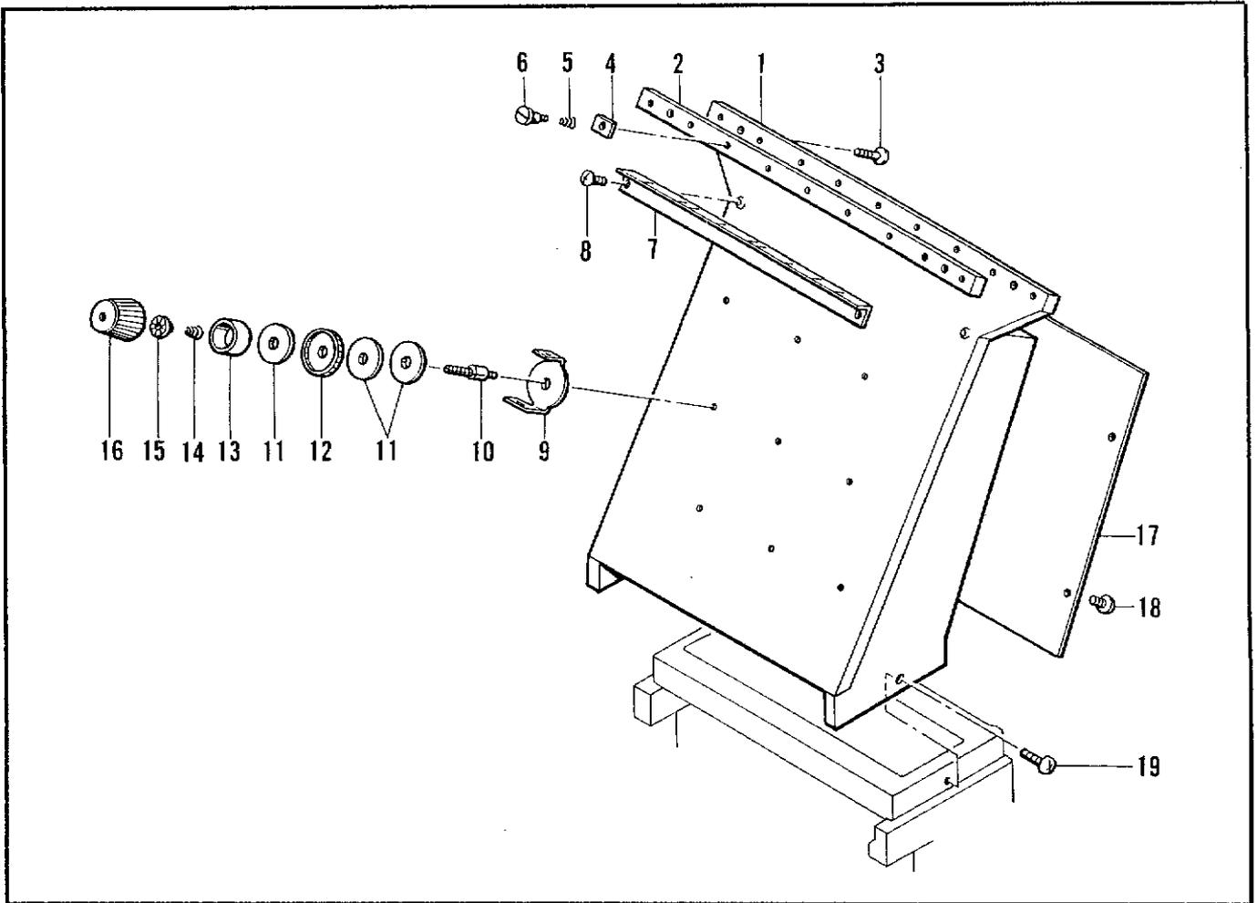
H. 上軸関係 / Upper shaft mechanism / Obere Welle /
