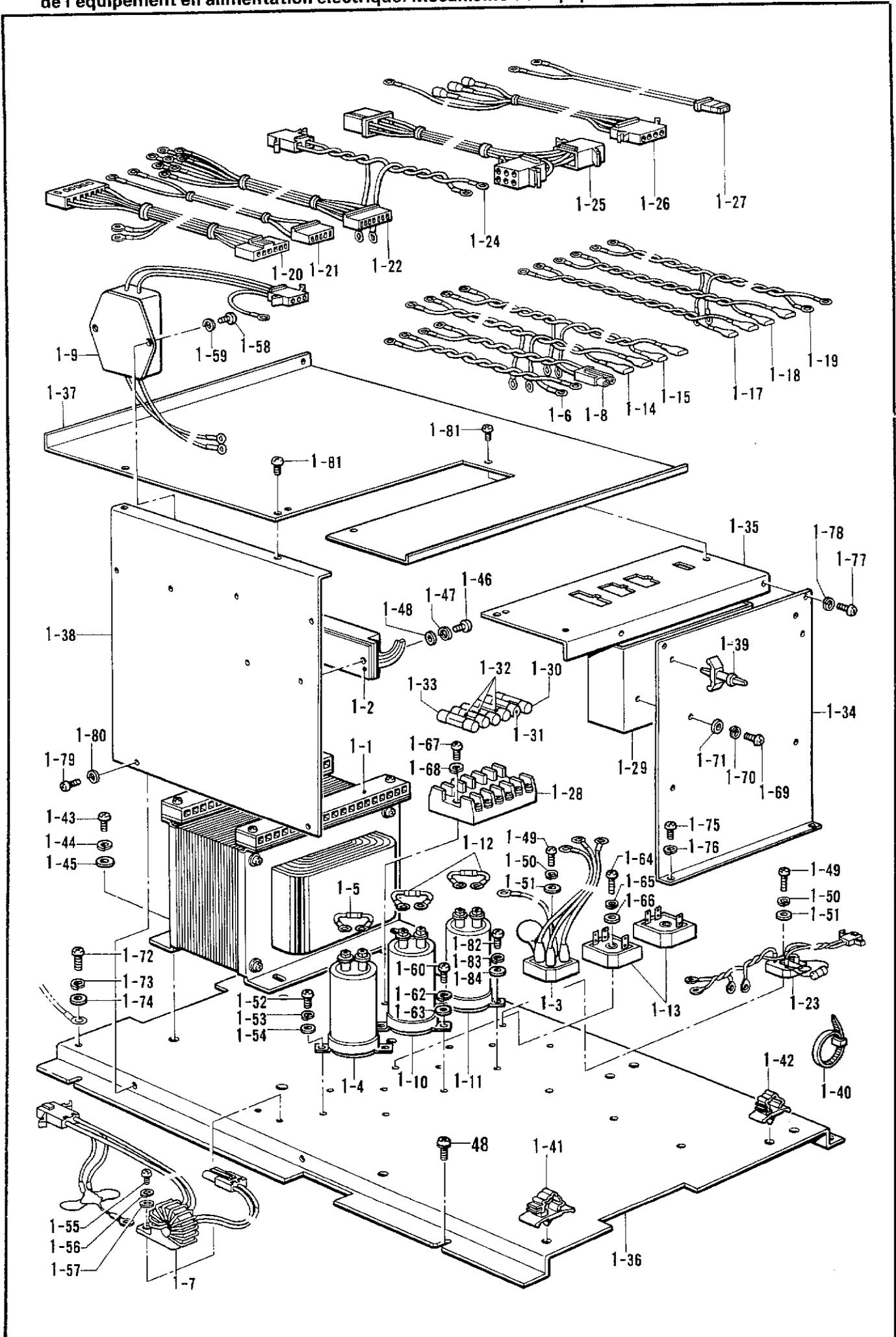
Q1. 電装品関係/Power supply equipment mechanism/Stromversorgung/Mécanisme
