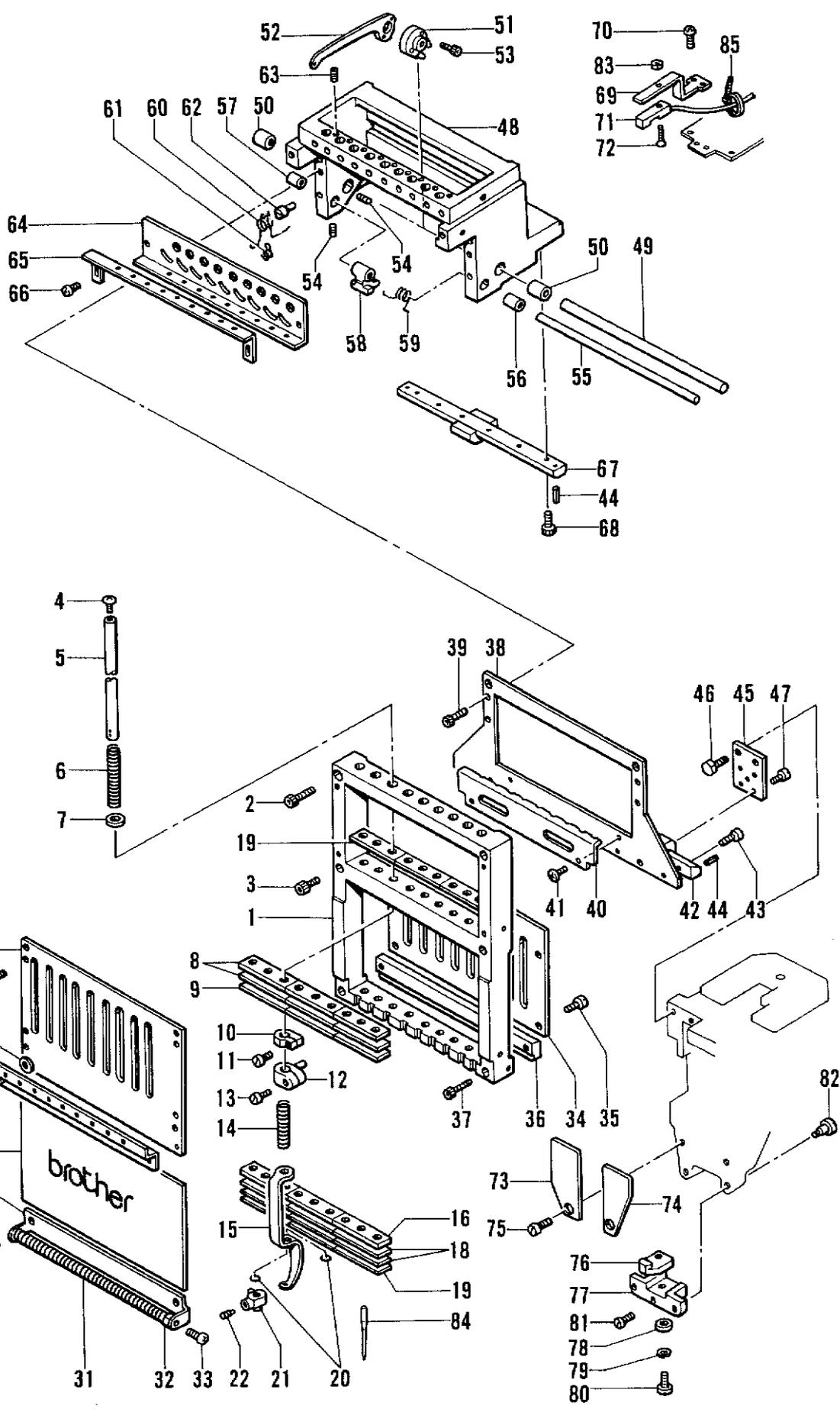
B. 針棒関係/Needle bar mechanism/Nadelstangenvorrichtung/
