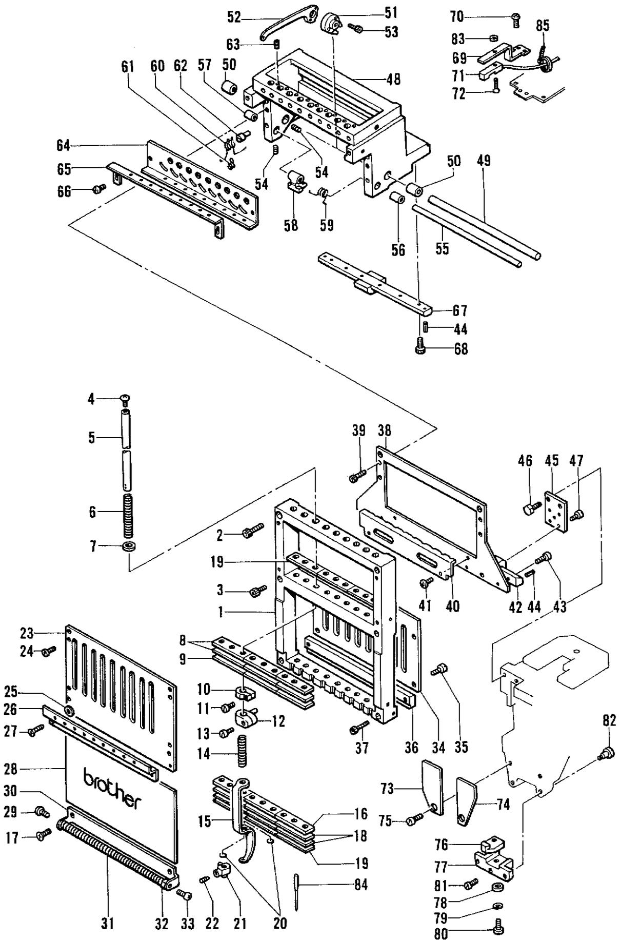
B. 針棒関係/Needle bar mechanism/Nadelstangenvorrichtung/
