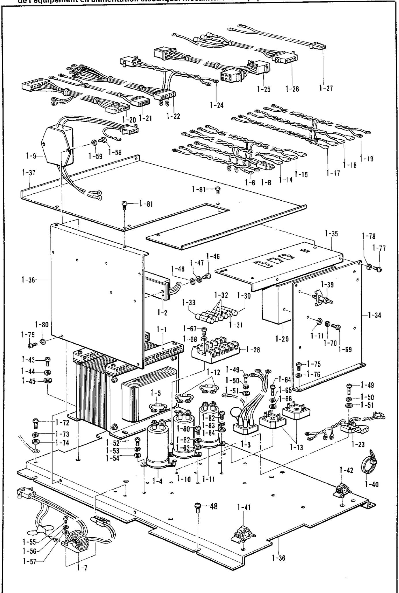
Q1. 電装品関係/Power supply equipment mechanism/Stromversorgung/Mécanisme
