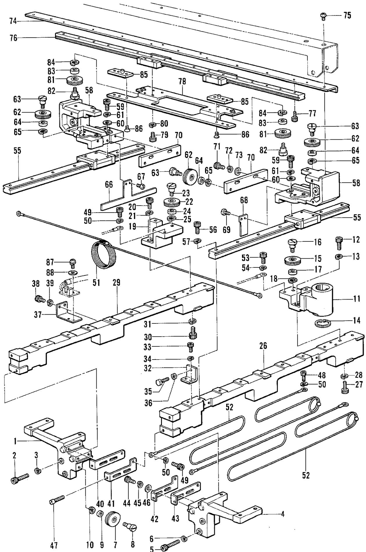
M. 送り・案内関係/Feed guide mechanism/Transportführung/
