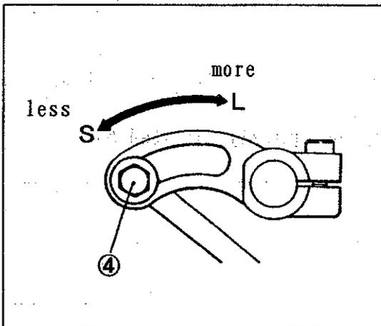
Up and down movement of top feed dog can be adjusted from 3.5 mm to 6.0 mm.
