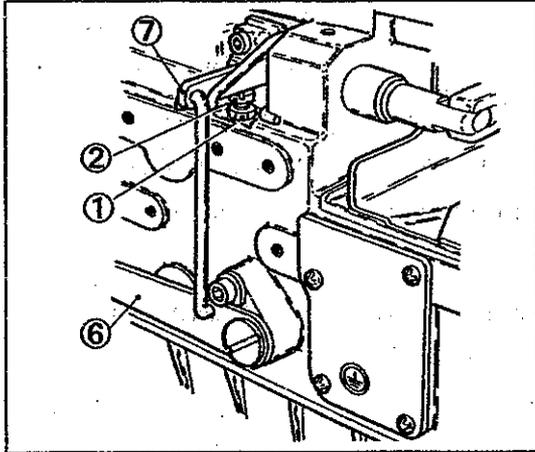
For AZR8920G, maximum lifting amount of presser foot is 3.5 mm.
