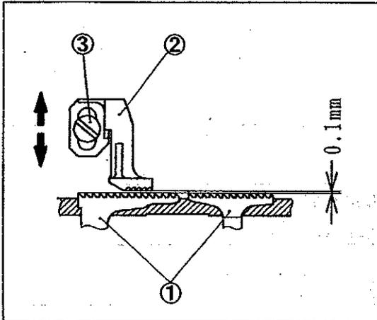
Stable feeding can be obtained by adjusting the height of top feed dog according to the application, type and weight of fabric to be sewn.
