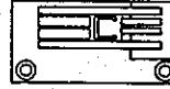
AS60-1784 - THROAT PLATE, 4.8MM AS60-1808 - THROAT PLATE, 5.6MM AS60-1785 - THROAT PLATE, 6.4MM SCREW - 22524
