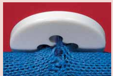
DAMAGE OF THE SEWING MATERIAL
