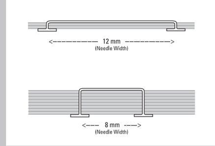
**Ensure perfect Plastic Staple fastener size** for every application. Needle spacing can be adjusted between .25” (6mm) and .5” (12mm).
